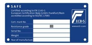
Below an example of a certification mark for an ATM safe III according to EN 1143-1 (with bar code):
